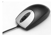
Vibrating mouse to alert user to take microbreaks
