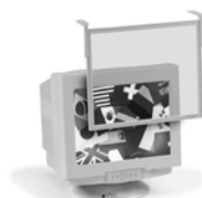
Anti-glare screen may help to enhance screen contrast and reduce eyestrain
